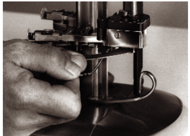
Figure 9. Adjusting Bevel Bloc Shoes
